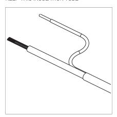
Step 7. Place 1" outer insulation tube over metal mesh shielding. Use a heat-gun or lighter, evenly heat tubing for 10 secs. This will cause tubing to shrink secure tubing over mesh shielding, to act as electrical insulation.
