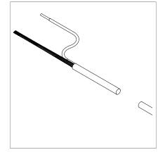
Step 2.Cut off excess wire length
