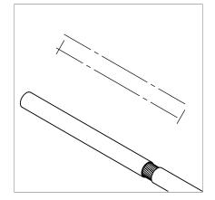
Step 4. Remove outer insulation tube to expose meshed metal shielding. MAKRE SURE TO KEEP THIS INSULATION TUBE
