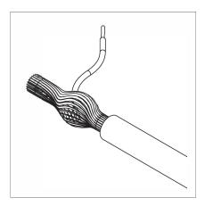
Step 5. Careful push to seperate metal mesh shielding to expose inner wire, take inner wire out from side of metal mesh shielding.
